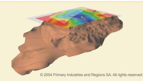
Gravity & magnetic data collected from the air, on the ground, and down-hole can be modelled in 3D with rock density and magnetic susceptibility constraints as well as other geoscience information. These efforts can help identify valuable and well-constrained drill targets to reduce exploration drilling risk.
